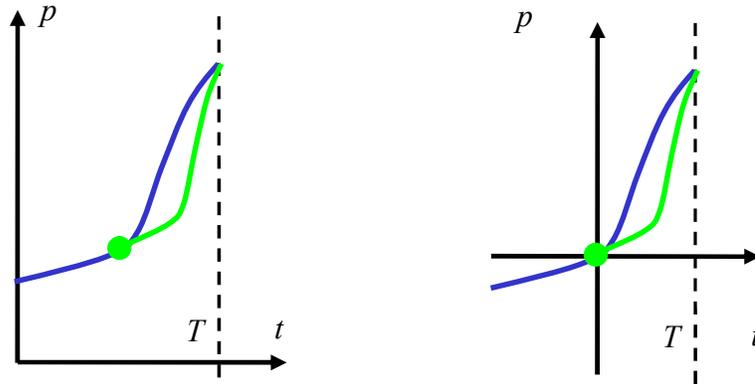
Figure 2 “Sliding” 2-point osculating interpolation of  $p(t)$
