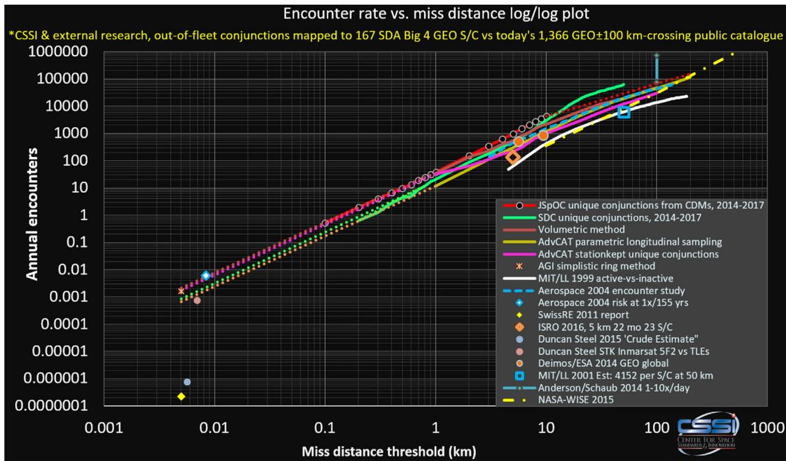
Fig. 60. Comparison of external and CSSI results for 167 SDA Big 4 operator satellites, including extrapolation via miss distance ratio power law (exponent = 1.85 below 1 km and 1.2 above 10 km).
