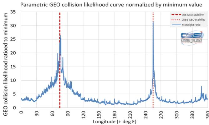
Fig. 52. AdvCAT parametric collision likelihood assessment height is similar to SwissRE flux-based approach, but peak-to-valley ratio of over thirty is much larger than the factor of seven originally noted in Ref. [8].
