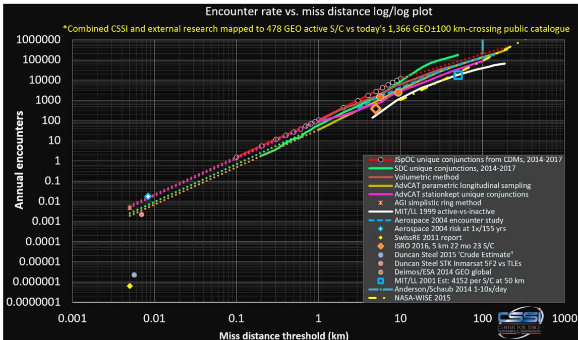
Fig. 61. Estimated GEO encounter rates for 478 active GEO ± 100 km satellites versus the 2017 RSO public catalogue.
