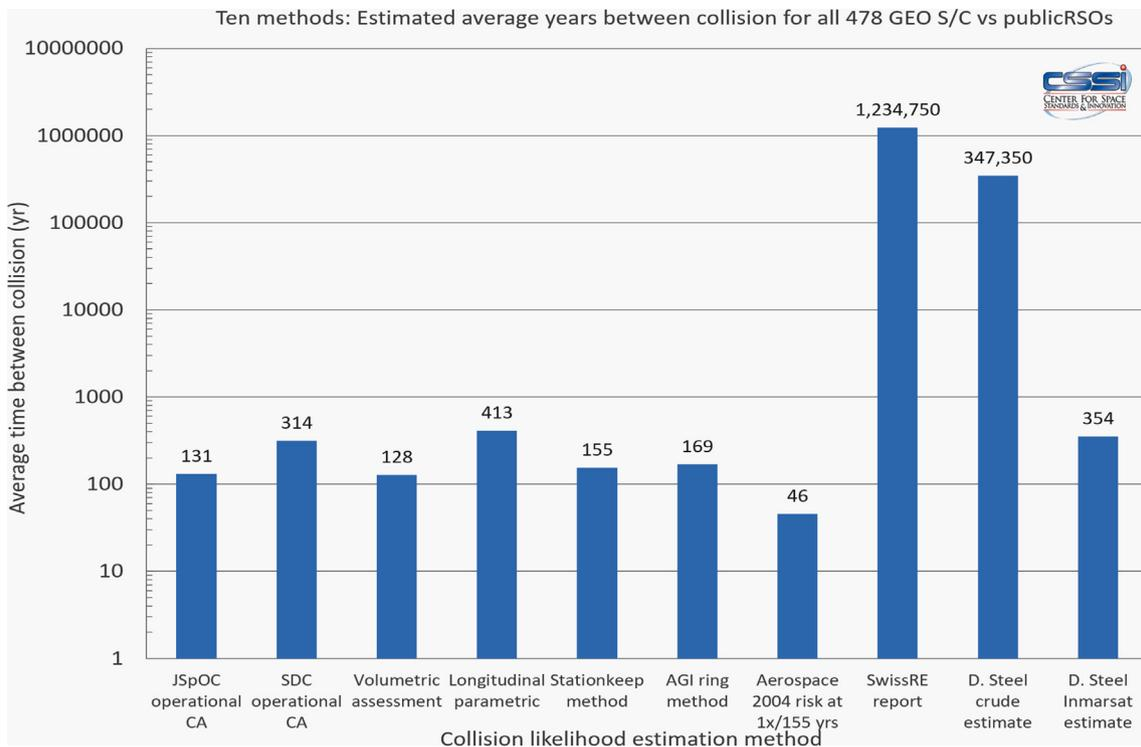
Fig. 62. Average years between collisions for 478 active GEO satellites versus the 2017 RSO public catalogue.
