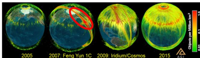
Fig. 43. A sequence of 3-Dimensional spatial density depictions of the public catalogue, including the red-encircled plus-up of the Iridium/Cosmos event. Such a non-longitude-averaged peak is much more pronounced than either 1D or 2D depictions could possibly indicate. (For interpretation of the references to colour in this figure legend, the reader is referred to the Web version of this article.)
