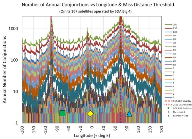
Fig. 50. AdvCAT parametric assessment of annual conjunctions vs longitude and miss distance threshold for Eutelsat, Inmarsat, Intelsat and SES' 167 spacecraft.
