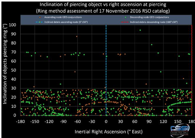
Fig. 23. Inclination of catalogued objects piercing a GEO ± 100 km ring vs right ascension.
