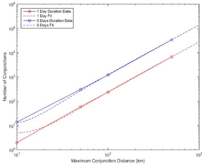
Fig. 32. “Number of conjunctions of the 2011 catalog with debris vs [minimum] conjunction distance in km for a 1-day time frame (red) and a 5-day time frame (blue)”. (included by permission of author). (For interpretation of the references to colour in this figure legend, the reader is referred to the Web version of this article.)
