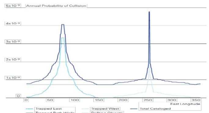
Fig. 27. Flux-based estimate of GEO collision likelihood [24] (included by permission of author).
