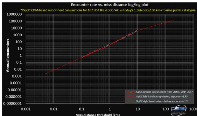
Fig. 47. Left- and right-hand extrapolation of 167 satellite trend using pre-computed power law exponents 1.85 & 1.2.
