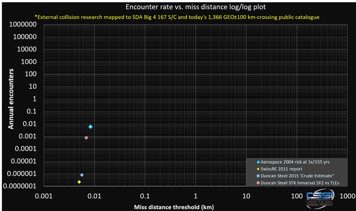
Fig. 28. Relevant external research on estimated collision likelihood, mapped to 167 “SDA Big 4” satellites and a 2017 JSpOC catalogue containing 1366 GEO ± 100 km-crossing RSOs.
