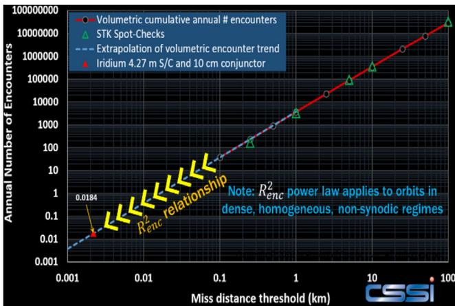
Fig. 35. Demonstration of encounter rate proportionality to  $R_E^2$  using the Iridium constellation (LEO).
