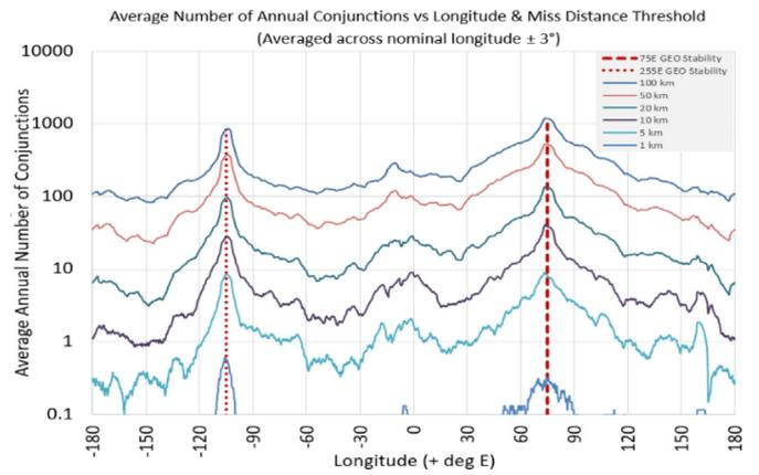
Fig. 53. Moving average filtered AdvCAT parametric assessment of annual conjunctions vs longitude and miss distance threshold for Eutelsat, Inmarsat, Intelsat and SES' 167 spacecraft.
