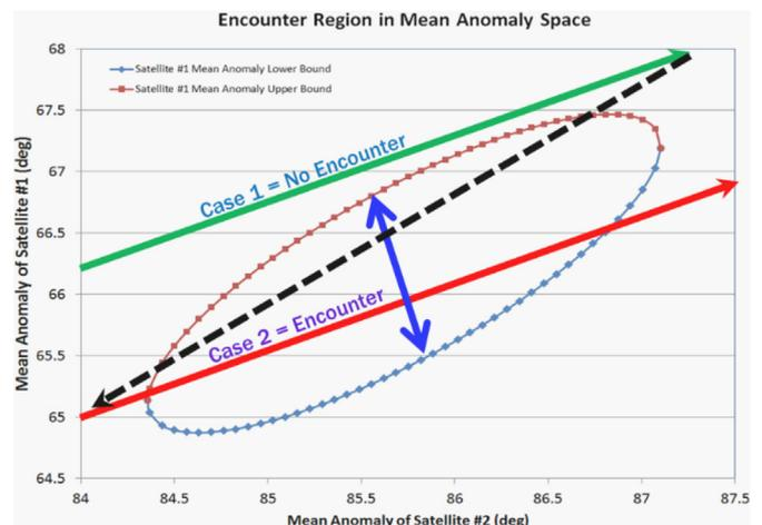
Fig. 34. Encounter geometry in mean anomaly space (representing constituent likelihood on a unit sphere).
