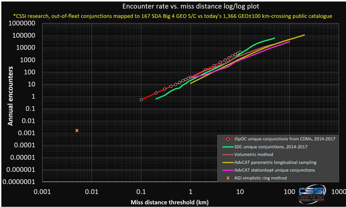
Fig. 59. Six CSSI GEO collision and/or encounter rate profiling techniques for 167 SDA Big 4 operator satellites.
