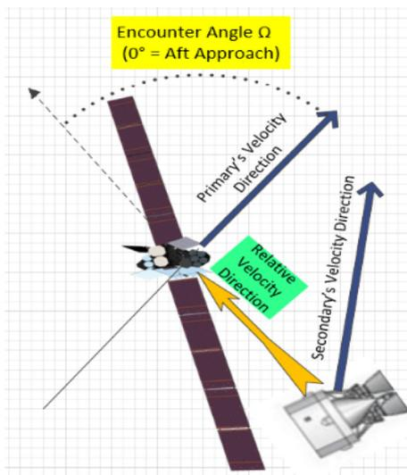
Fig. 11. Close approach relative velocity encounter angle.
