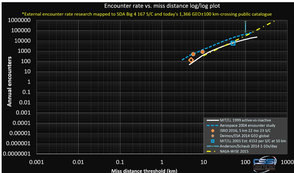
Fig. 33. Relevant external research characterizing estimated encounter rate, mapped to 167 “SDA Big 4” satellites and a 2017 JSpOC catalogue containing 1366 GEO ± 100 km-crossing RSOs.
