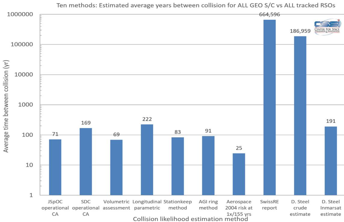
Fig. 64. Average years between collisions for all active GEO satellites vs all tracked RSOs.
