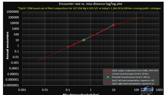
Fig. 49. Comparison of number of encounters at current and potential CA quality levels.
