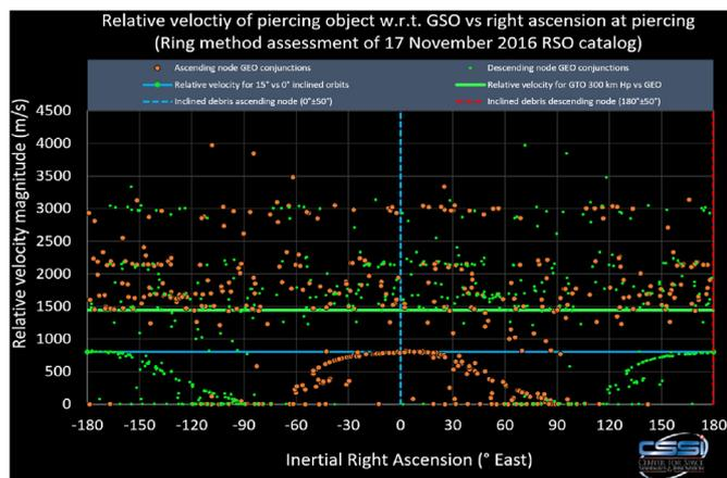
Fig. 22. Relative velocity of catalogued objects piercing a GEO ± 100 km ring vs right ascension.
