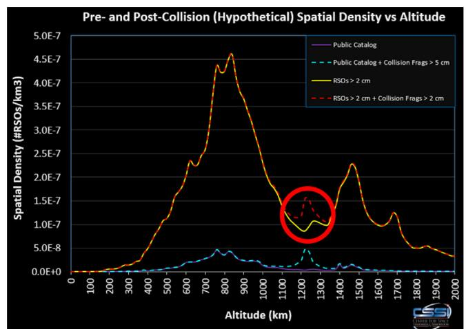
Fig. 41. 1-Dimensional spatial density =  $f(\text{altitude})$ , showing trends matching the public catalogue, estimated 2 cm catalogue, and a plus-up (red dotted hump at 1200 km) after a hypothetical fragmentation event. (For interpretation of the references to colour in this figure legend, the reader is referred to the Web version of this article.)
