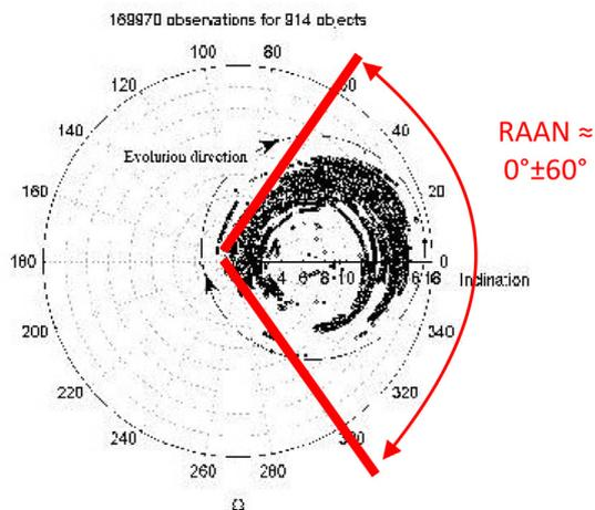
Fig. 20. Inclination vector in phase space for 914 GEO RSOs (Fig. 4.4 from Ref. [20], included by permission of author).
