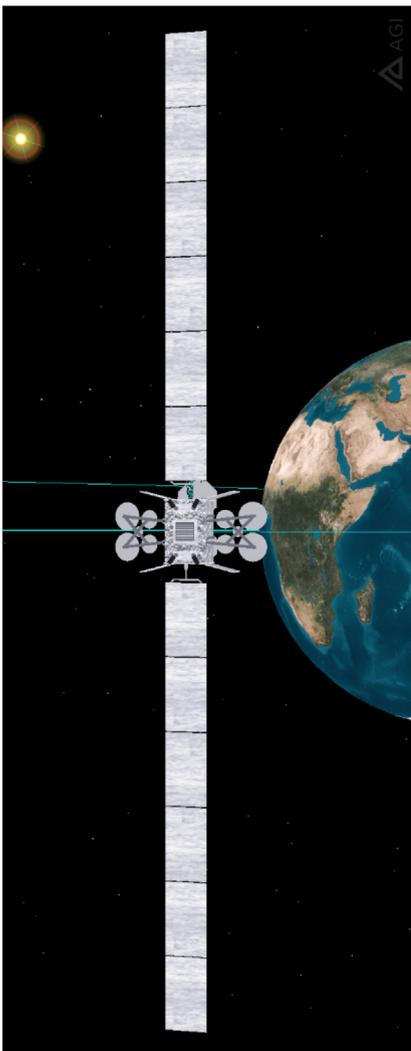
Fig. 8. Boeing 702 satellite, viewed from above (nearly normal to solar panels).
