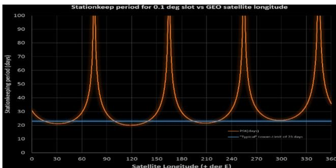
Fig. 57. Typical stationkeeping period vs longitude.
