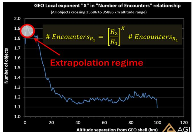
Fig. 40. Combined [altitude + unit sphere] exponent in the neighbourhood of the GEO altitude shell, with an average of 1.85 within 10 km of GEO.
