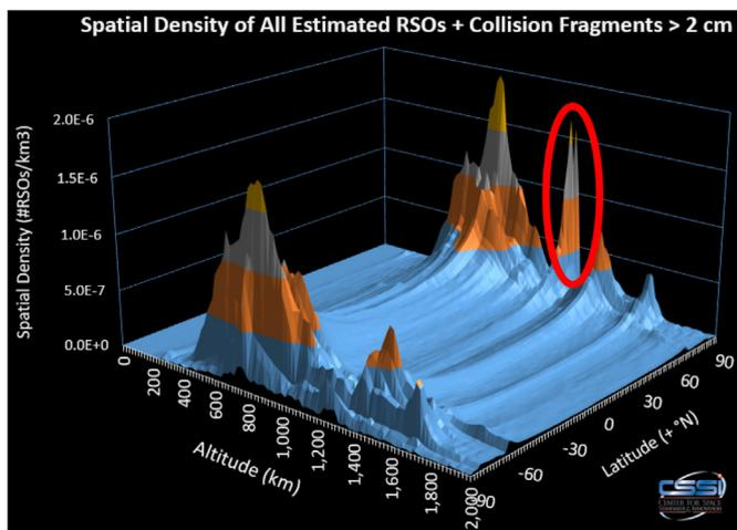
Fig. 42. 2-Dimensional spatial density for the estimated 2 cm catalogue, including the plus-up (red encircled hump at 1200 km) after a hypothetical fragmentation event. Note that this non-latitude-averaged peak is dramatically more pronounced than the 1D depiction indicates. (For interpretation of the references to colour in this figure legend, the reader is referred to the Web version of this article.)
