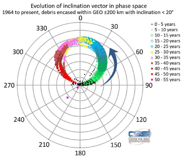
Fig. 21. Refresh of Nazarenko’s inclination vector in phase space for period 1964 to present, all debris encased by GEO ± 200 km with inclination < 20°. Colours denote how far into cycle the RSO’s evolution was at that time. (For interpretation of the references to colour in this figure legend, the reader is referred to the Web version of this article.)
