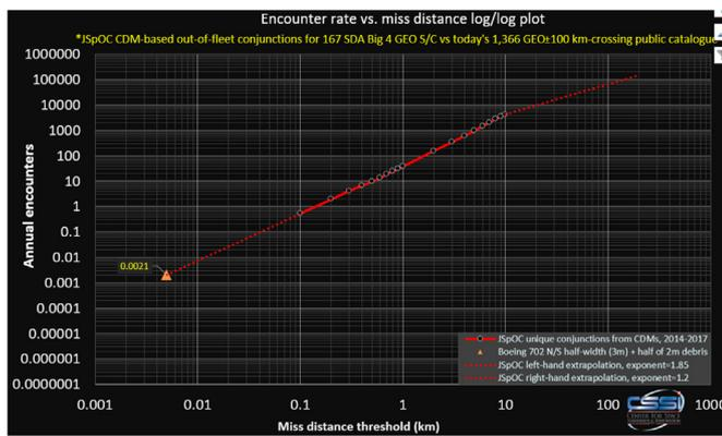
Fig. 48. Extrapolation of encounter rate trends permits estimation of hardbody collision likelihood (0.0012 annually for these 167 satellites).
