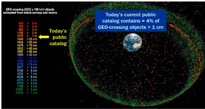
Fig. 3. Estimated GEO-crossing objects > 1 cm in GEO ± 100 km altitude vs the 2017 1366 RSO GEO-crossing public catalogue.
