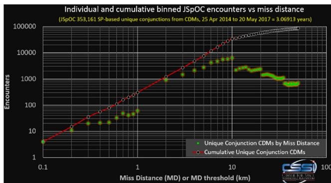
Fig. 45. Assembly of JSpOC CDM-based “cumulative annual GEO unique encounters” trend in log/log space.
