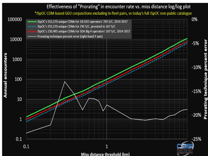
Fig. 44. Effectiveness of “prorating technique” used for mapping disparate collision and encounter rate profiles.
