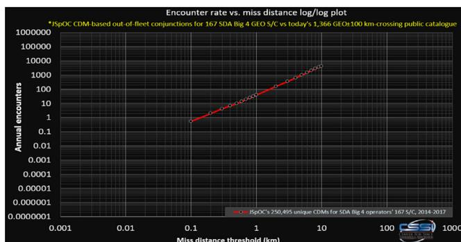
Fig. 46. Assembly of JSpOC CDM-based “cumulative annual GEO unique encounters” trend in log/log space.
