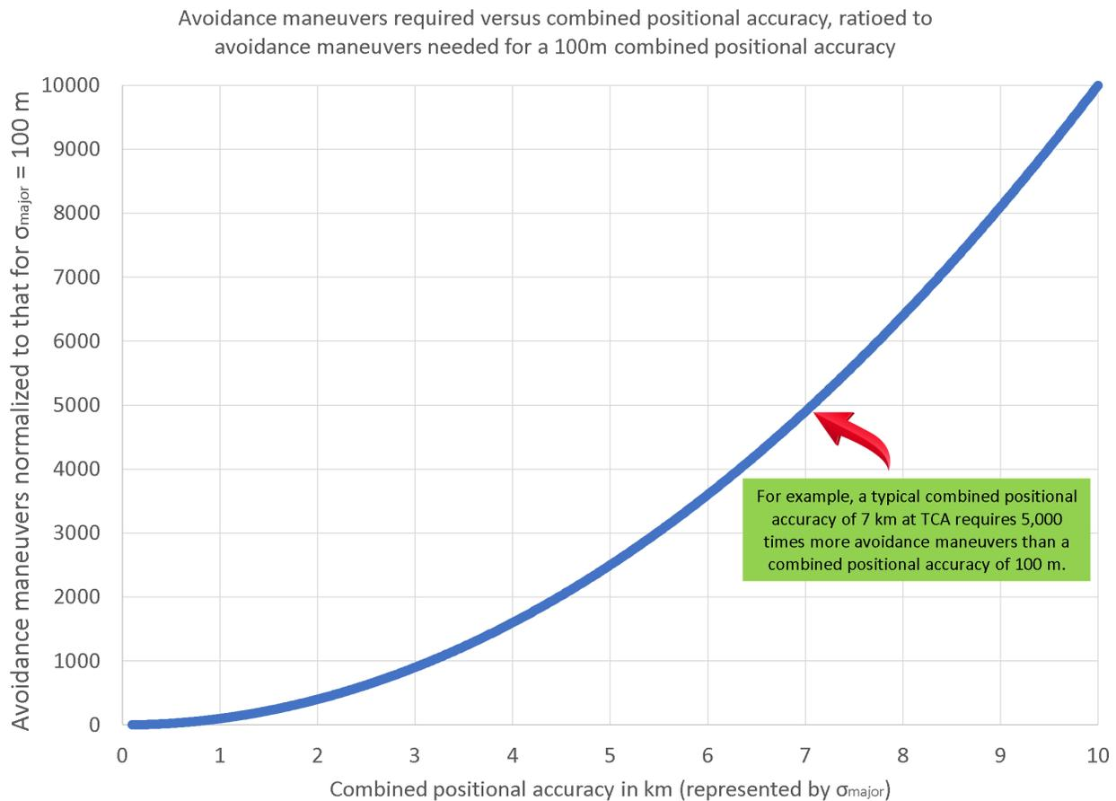
Figure 17. Encounter rate increase as a function of combined positional accuracy for distance-based screening.
