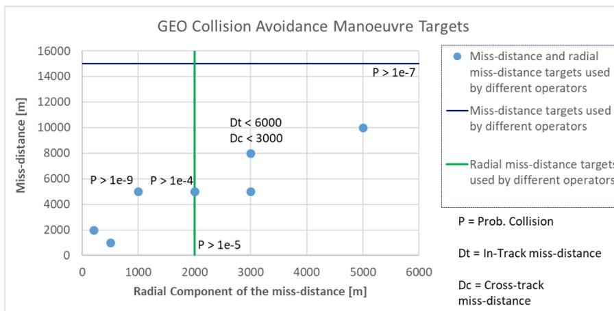
Figure 7: GEO Collision Avoidance Maneuver Targets
