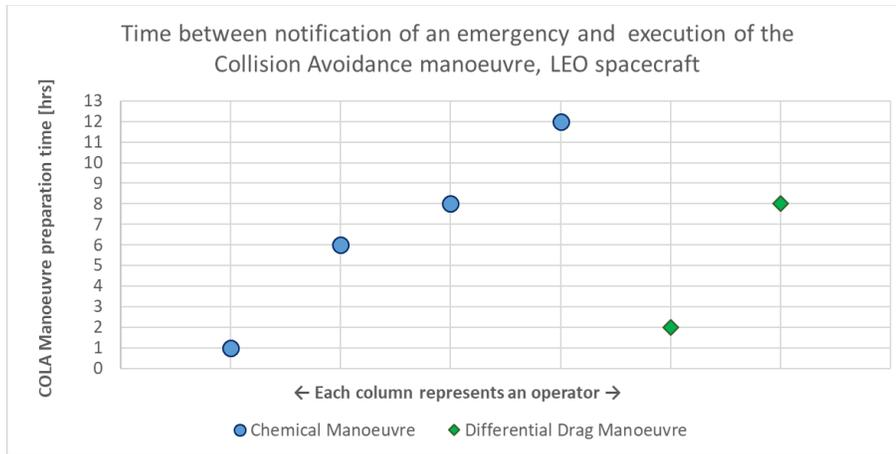
Figure 6: LEO Reaction Time
