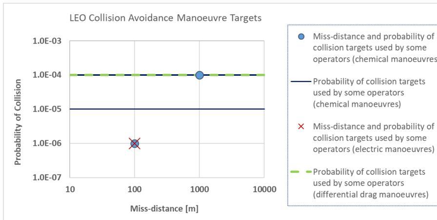
Figure 8: LEO Collision Avoidance Manoeuvre Targets
