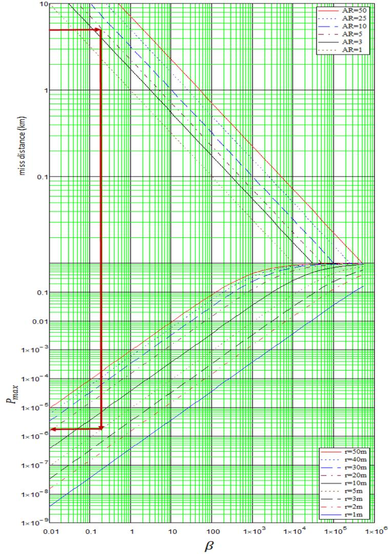
Figure 15. Example of using linked nomograms to determine  $P_{max}$  from  $r$ ,  $d$ , and  $AR$ .
