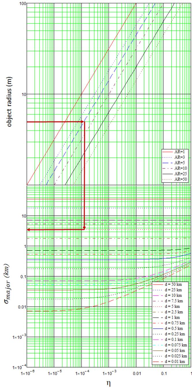
Figure 16. Nomogram to determine  $\sigma_{major}$  from  $r$ ,  $d$ , and  $AR$ .
